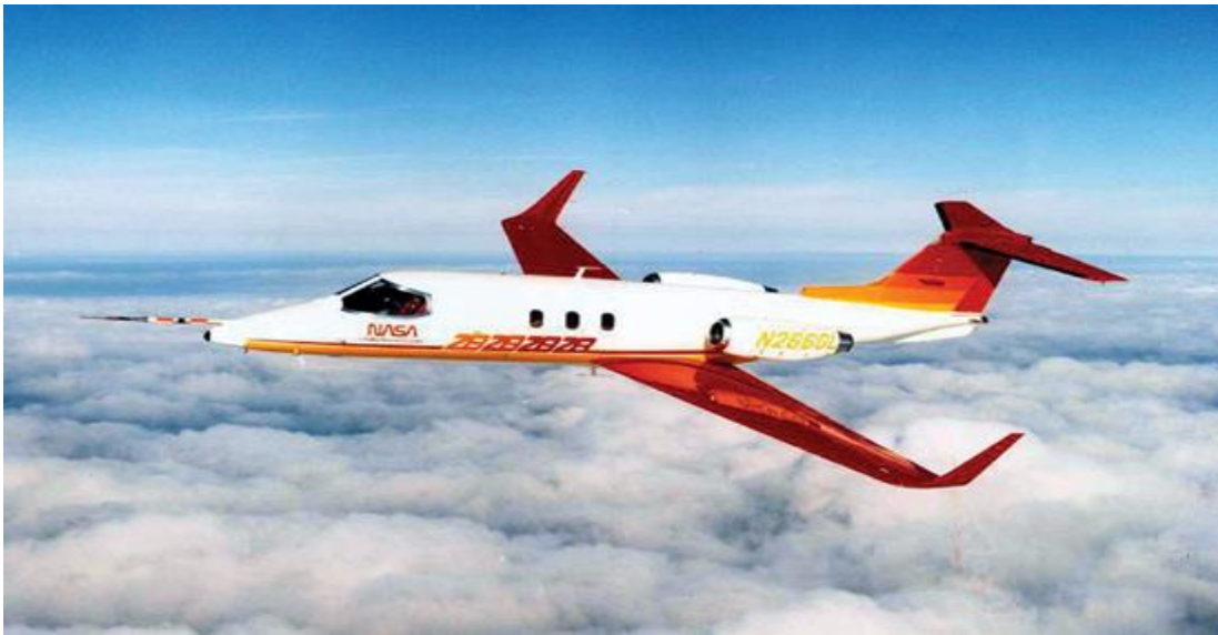
Figure 23, A Learjet aircraft with winglets
