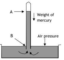
The first force is due to the weight of mercury - this drags the mercury down the tube into the beaker. The second force is due to the air pressure on the surface of the mercury in the beaker, which tries to push it back up the tube. Sooner or later the two forces will balance and the mercury will settle at a certain height (marked A on the diagram).
