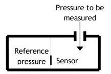
Finally this gauge is also easy to modify to measure differential pressure:
