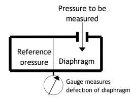
Instead of an analogue meter, the deflection of the diaphragm can be measured with an electronic sensor. This can be a simple strain-gauge, a piezoelectric deflection sensor or a capacitive sensor:
