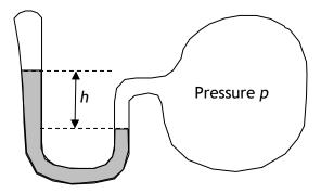
More often in engineering, a manometer is rigged up so read differential pressures (differences in pressure ( $\Delta p$ ) between two points), for example in a pipe.
