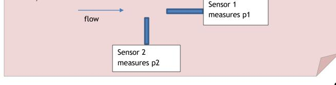
You may also see the term "stagnation pressure" used in some books. This is essentially the same as the total pressure defined above (it's defined as the (static) pressure measured when a moving flow has been brought to a complete to a complete halt).
