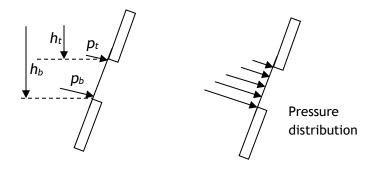
Because the depth of water at the bottom  $(h_b)$  is greater than that at the top  $(h_t)$ , we must be careful to take this into account in any design. To calculate the total force on the window, we have to integrate the force over the whole area (although, to be on the safe side, we could just assume that the force on the bottom was the present over the whole area). For a window like this one, the result turns out to be.
