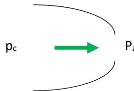
In the rocket of course  $p_c$  would be combustion-chamber pressure and  $p_a$  would be the ambient (air) pressure at the exit.
