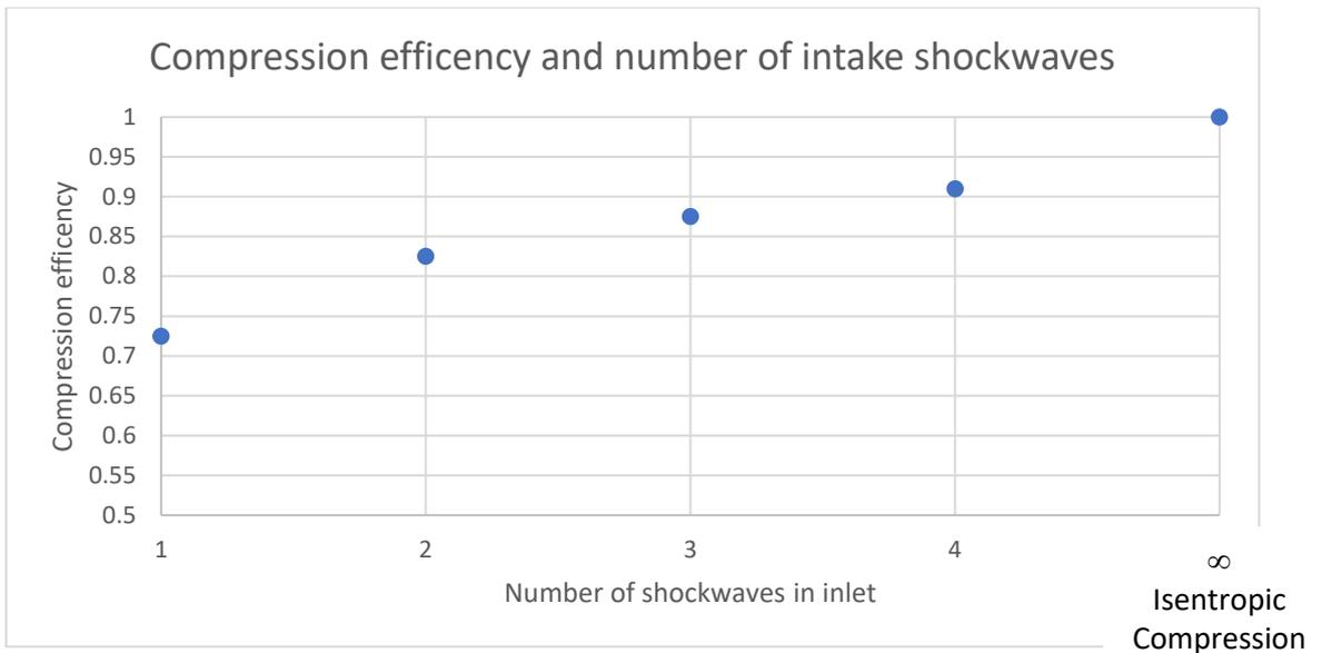
This limiting case is known as an *Isentropic Compression Surface* and is a gently curved surface which compresses the flow gradually. Unfortunately, detailed design of this surface is somewhat involved, and we don't have time to cover it in here.
