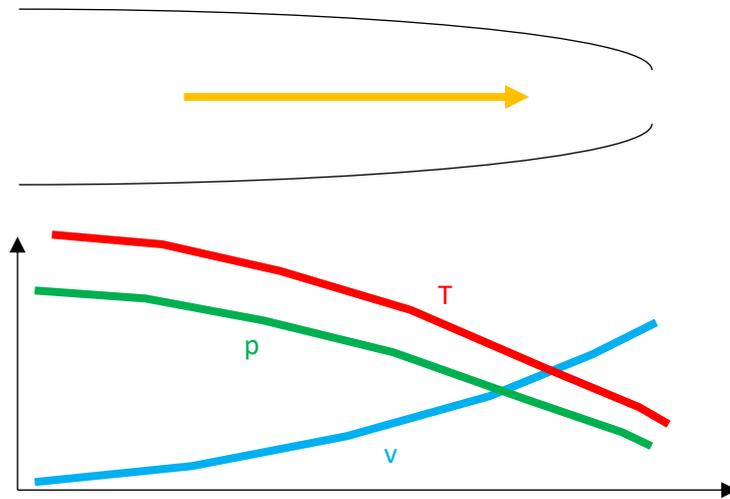
Eventually, if we increase the pressure difference enough, the Mach number at the throat will reach one ( $M = 1$ ) and we can't go to any higher velocity - because, above Mach 1 speed decreases in a converging duct (eqn 0). The pressure ratio necessary to give this condition is given by setting  $M = 1$  in equation 2 and the mass flow-rate is given by setting  $M = 1$  in equation 4.
