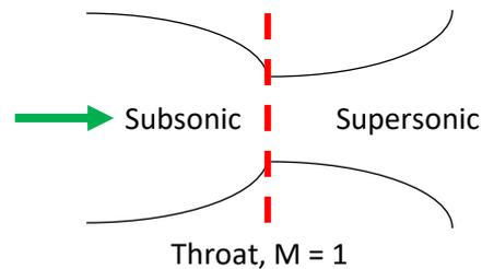
Where the constriction in the centre is called the throat and must have a Mach number of 1 if the flow is to continue to accelerate (and a normal shockwave must therefore be present here).
