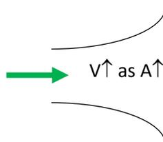
Therefore, the area–velocity relationship tells us that subsonic and supersonic flow behave in exactly the opposite way (with regard to velocity) in ducts.
