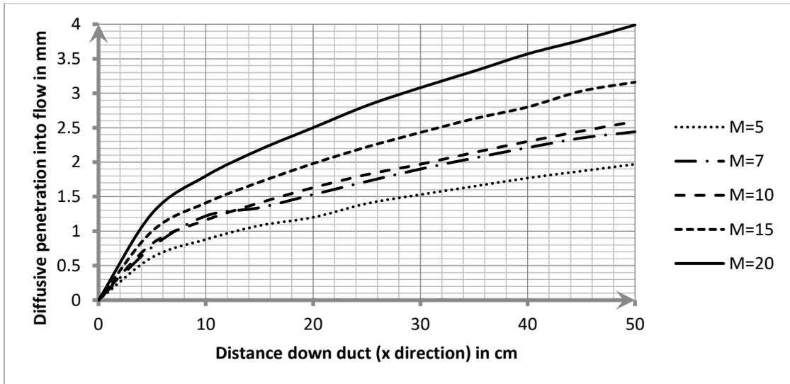
As can be seen, by the time the flow moves down the duct by, for example 25cm, the penetration is only a few millimetres.
