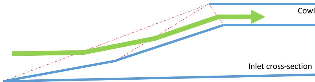
The red dotted lines are the shockwaves, the blue lines are a cross-section of the inlet (which in this case is a linear inlet, like that shown in the diagram on page 1 - but this representation is up-side down compared to that diagram). The green arrow is the airflow.
